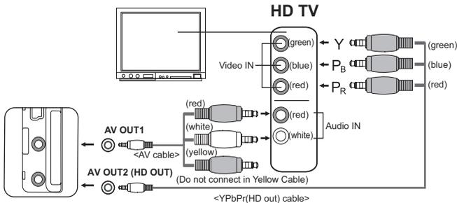
1. Connect one end of the YPbPr (HD out) cable into the (Video IN) port on the HDTV and the other end into the AV OUT2 (HD out) terminal of the digital video camera.
